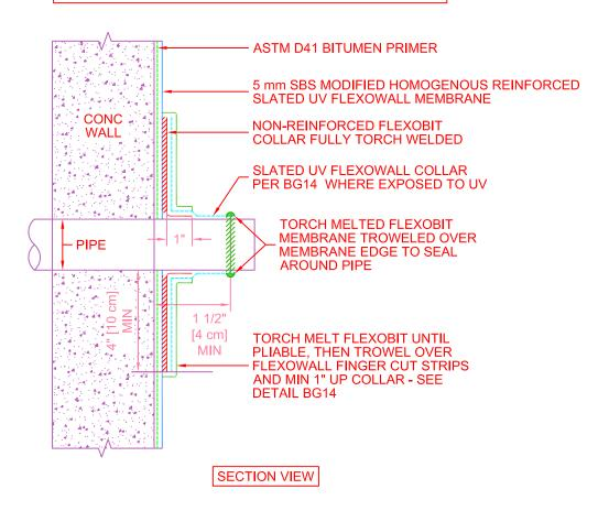
PIPE PENETRATION AT WALL (WITH UV EXPOSURE)
